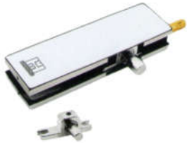
DAT-304 Glass door clamp Material: Stainless steel Finishing: Chrome finish/Sain finish/Gold finish Door thickness: 10-12mm Tempered glass
